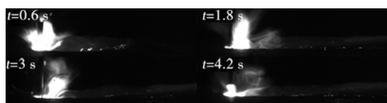
图 7 80% Ar-20% \text{CO}_2 气体保护,熔池高速摄影照片 Fig. 7 High speed photographs of weld pool with 80% Ar-20% \text{CO}_2 shielding gas
