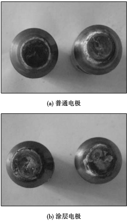
图 7 普通电极和涂层电极失效后端面宏观形貌 Fig. 7 Appearance of uncoated and coated electrodes after failure
