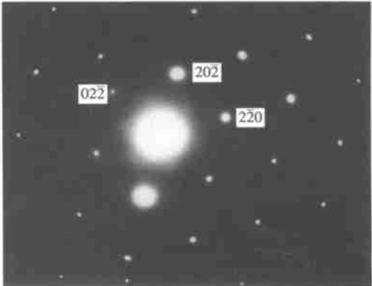
(b) [111] orientation electron diffraction pattern of Al
