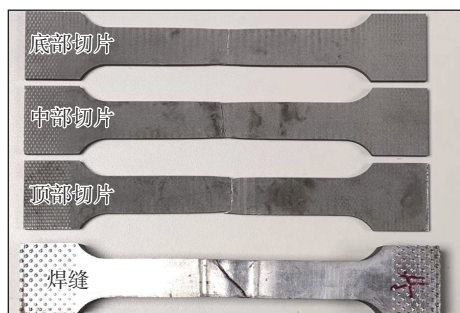
图 5 焊缝和焊缝切片拉伸试样 Fig. 5 Weld and welds slices specimens
