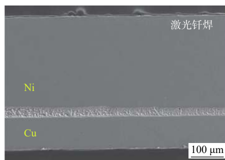
(c) 激光钎焊宏观形貌
