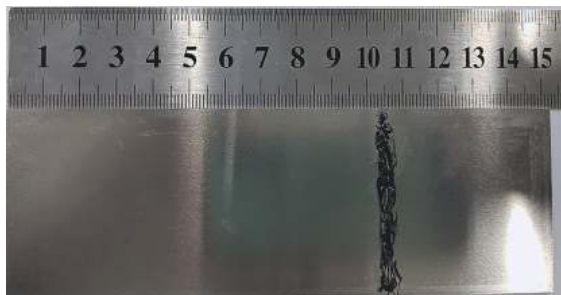
图 6 表面带有油污的试样 Fig. 6 Specimen with greasy surface
