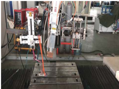
图 2 大气环境下激光焊接试验 Fig. 2 Laser welding test under atmospheric environment
