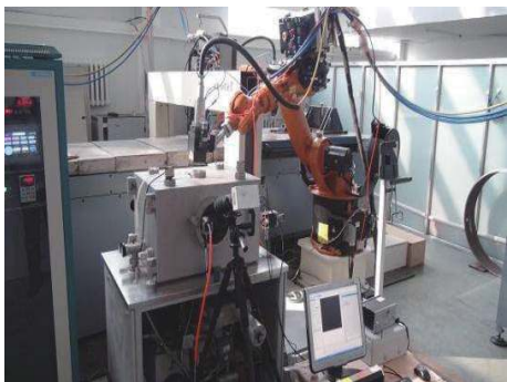
图 3 真空环境下激光焊接试验 Fig. 3 Laser welding test under vacuum environment
