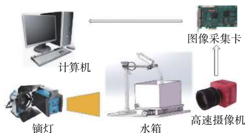
图3 高速图像采集系统图 Fig. 3 High-speed image acquisition system diagram
