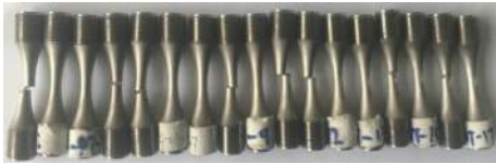
图 8 TC4-DT/TC21 接头高周疲劳性能试样 Fig. 8 Fatigue specimens of TC21+TC4-DT IFW joint
