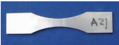
图 1 静轴肩搅拌摩擦 6005 铝合金接头疲劳测试试样 Fig. 1 Fatigue test sample of 6005 aluminum alloy joint after stationary shoulder friction stir welding
