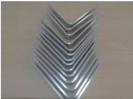
图 4 静轴肩焊接 6005 接头的正弯和背弯试样 Fig. 4 Face and root bending test of 6005 AA joint after stationary shoulder friction stir welding
