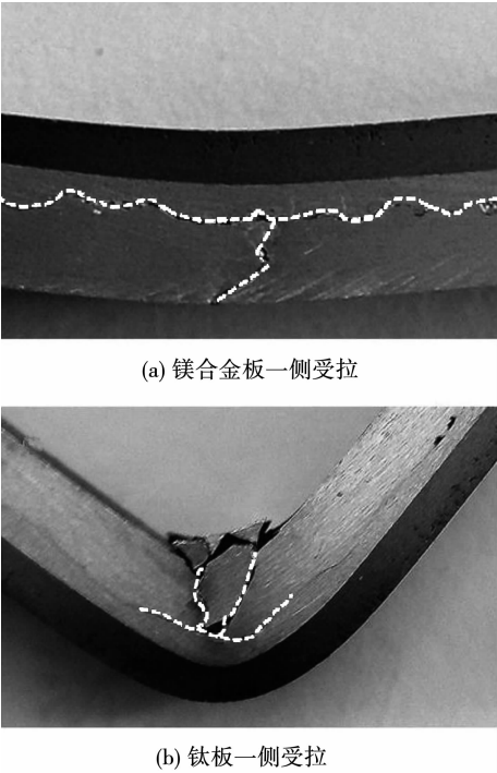
图 7 钛/铝/镁爆炸复合板弯曲试验前后试样的宏观形貌 Fig. 7 Photograph of Ti/Al/Mg explosion cladde plate after three-point bending test
