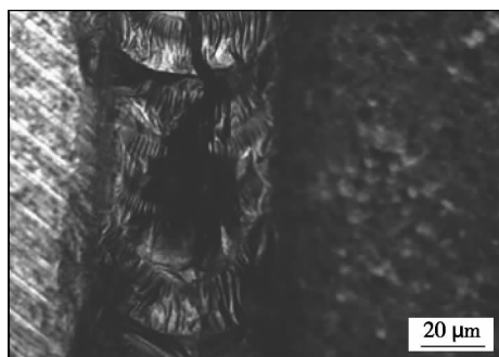
图 7 加工盖板缺口引起激光焊接接头裂纹 Fig. 7 Crack caused by Machining defects
