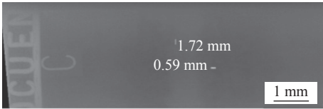
图 4 90°样品 RT 图像线性气孔 Fig. 4 RT film of sample 90° linear porosity
