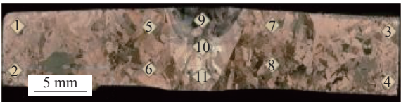
图 6 沿试样剖面的显微硬度测试点 Fig. 6 Microhardness points along sample profile
